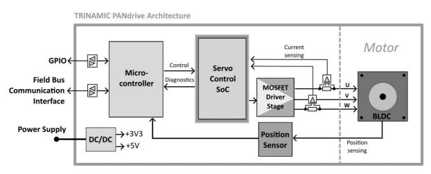
Figure 4 – Top-level block diagram of a PANdrive™ smart motor solution by Trinamic.
