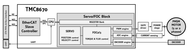
Figure 3 – Top-level block diagram of the TMC8670 shows the different blocks that are all combined in one single motor driver chip, such as communication and FOC in hardware.
