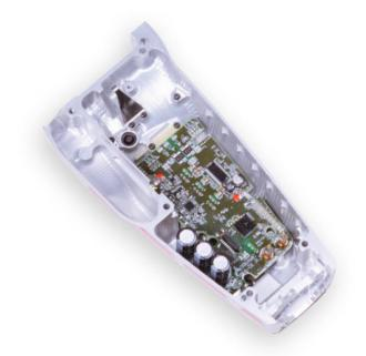
Figure 1 – Miniaturized PCB custom-made for a perfect fit in Össur's Power Knee, a battery-powered prosthetic leg.
