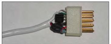
Figure 2. DB9 connector with embedded TO92 1-Wire device before injection molding.
