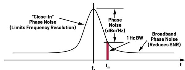
Figure 1. Phase noise of a nonideal sine wave.
