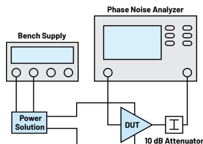
Figure 4. Simplified block diagram of the test setup used in the experiment.
