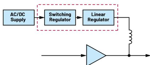
Figure 3. Power supply topology in an RF signal chain.
