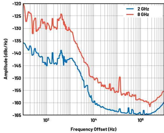
Figure 6. Phase noise response of the HMC8411 with the LTM8063, showing phase noise/frequency relation.
