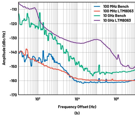
Figure 5. (a) HMC8411 and ADPA9002 performance at 2 GHz, and (b) phase noise response of ADPA9002 powered by the bench and the LTM8063 at two different input frequencies.
