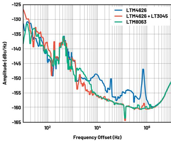
Figure 8. Phase noise response of the HMC8411 with various power solutions.  $f_c = 5$  GHz.
