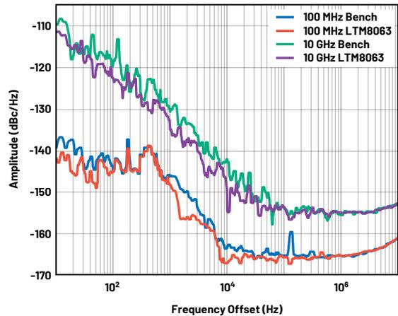
Figure 7. Phase noise response of the HMC8411 powered by the bench and the LTM8063 at two different input frequencies.
