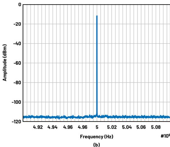
Figure 9. (a) Phase noise response of the HMC8411 at 5 GHz powered by different switching regulators, and (b) spectrum of the HMC8411 powered by the LTM4626 showing no spurs.
