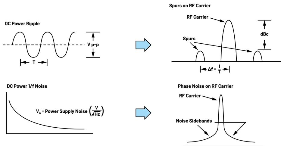
Figure 2. Noise on power rails and its effect on the RF carrier signal.
