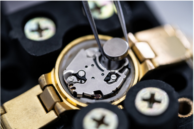
Figure 3. Silver oxide batteries are commonly used as watch batteries.
