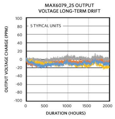
Figure 2. LTD plot for ceramic package.
