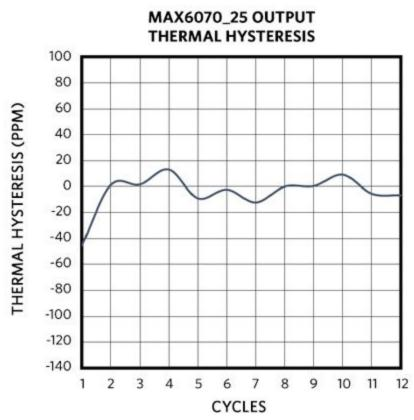
Figure 9. Typical thermal hysteresis plot.
