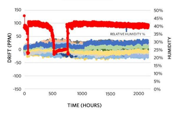
Figure 11. MAX6279 ceramic test chip LTD with regard to relative humidity.
