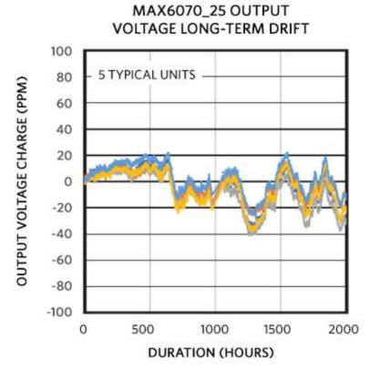
Figure 1. LTD plot for SOT-23 package.
