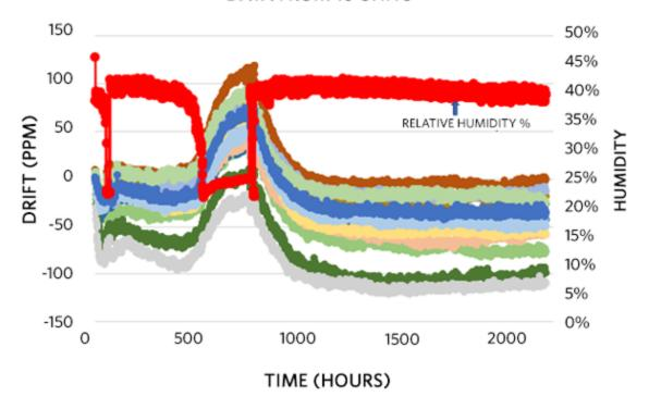
Figure 10. MAX6138AEXR25 (SC70-3 plastic package); LTD with regard to relative humidity.
