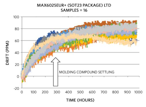
Figure 7. Package compound settles during the first 200-300 hours.
