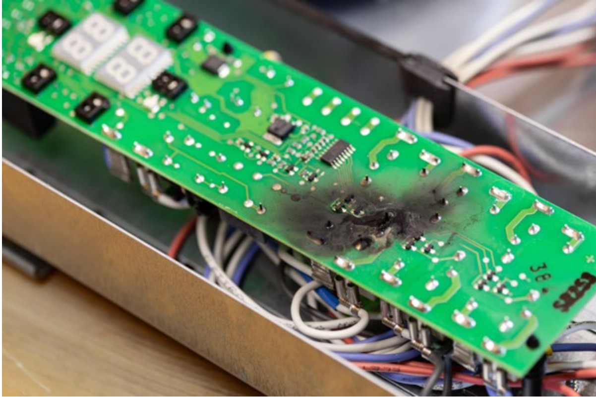
Figure 4. Board burned due to short circuit.
