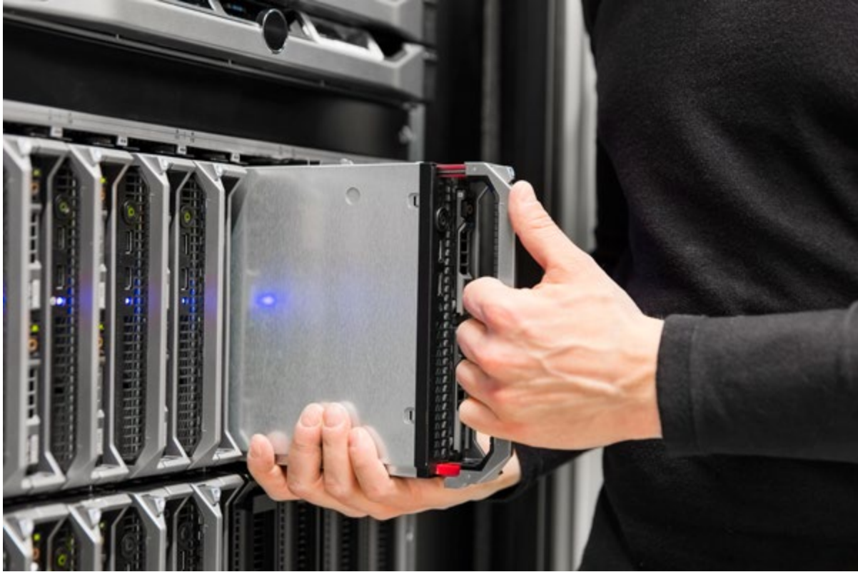
Figure 3. Hot swapping a system card.
