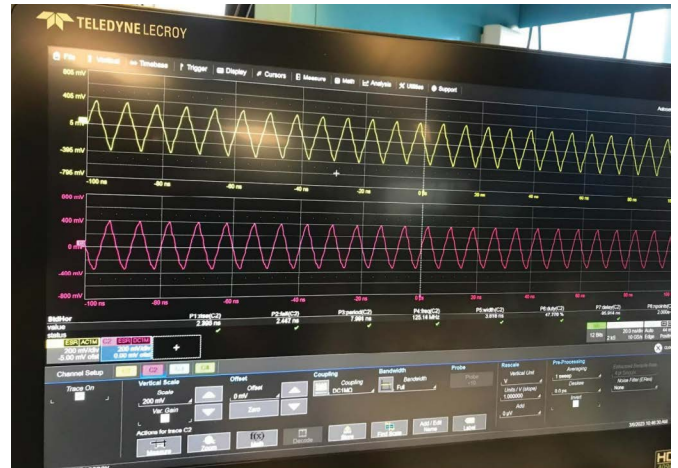
Figure 6. Optimized clock signal generated from the modified adaptor board going to each of the HTOL device under stress, eight of them without attenuation or clock jitter.
