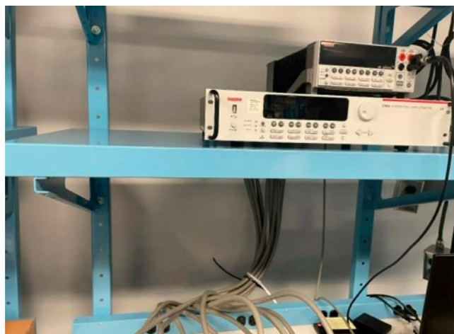
Figure 4. Typical lab setup for continuity testing of the integrated circuit
