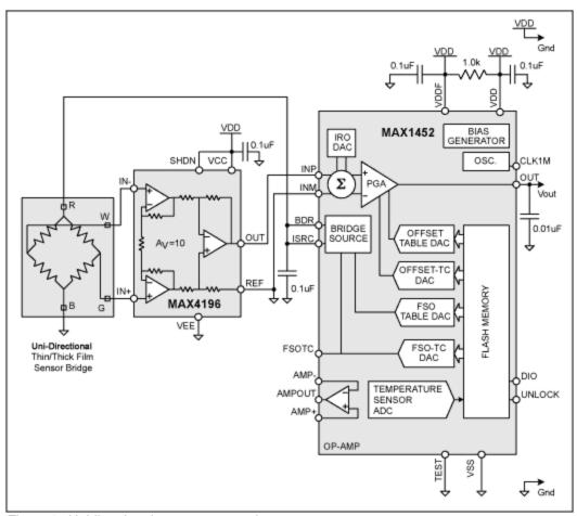
Figure 2. Unidirectional sensor connections.
