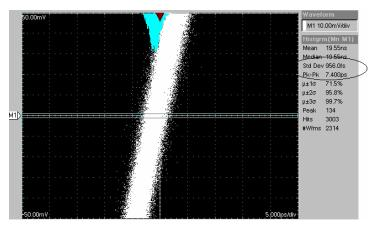
Figure 6. Random Jitter Measured with Improved Method
