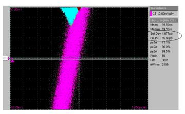
Figure 5. Random Jitter Measured in the Traditional Method
