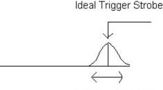
∆t trigger delay jitter
