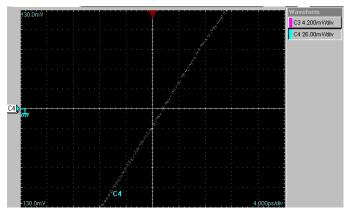
Figure 3. Finding the Slew Rate
