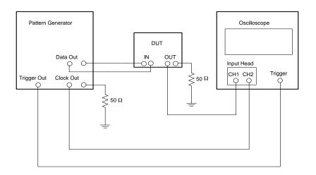
Figure 4. Configuration for Proper Measurement of Random Jitter
