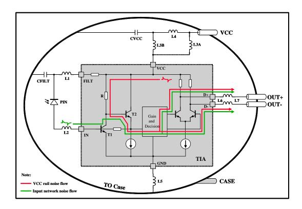
Figure 2: Simplified Equivalent Circuit of TIA and ROSA Assembly
