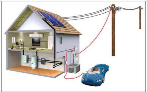
Figure 4. G3-PLC communication route from EV to utility.
