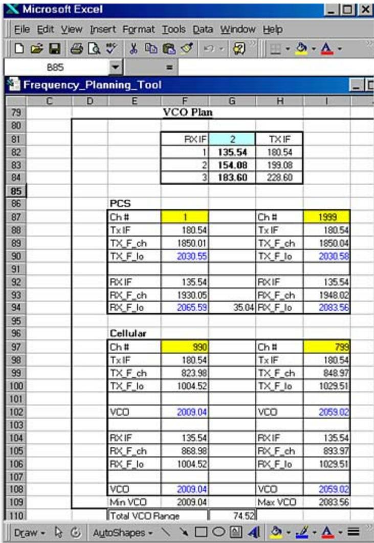
Figure 2. The maximum tuning range of VCO is calculated.
