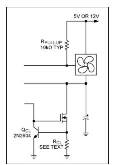
Figure 2. When current limiting is necessary for pass transistors, this circuit provides that function.
