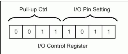
Figure 3. I/O control register configuration.
