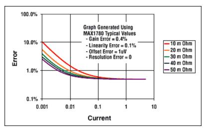
Figure 3. Coulomb-counter accuracy as a function of current and R<sub>SENSE</sub>.
