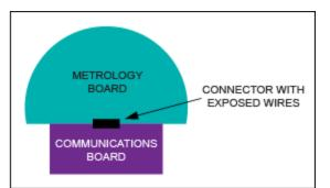
Figure 1. A two-board meter with unsecured metrology has data passing over exposed connector wires.
