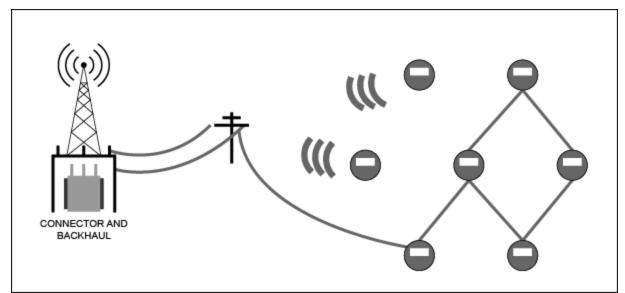
Figure 3. An AMI architecture has meters communicating by PLC or RF to a concentrator. Backhaul from the concentrator often occurs over the cellular network. Note that the ratio of meters to concentrators is greatly reduced in this graphic.
