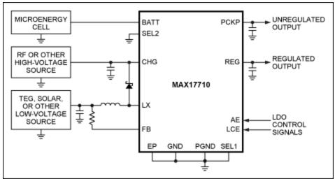
Figure 2. The MAX17710 shown in a typical application circuit harvesting from high-voltage charge sources.
