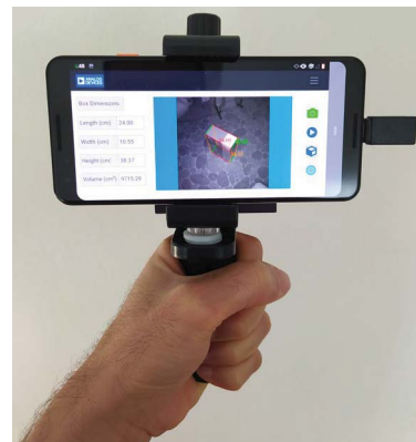
Figure 10. A handheld device integrated with 3D object dimensioning using the ADI ToF sensor.
