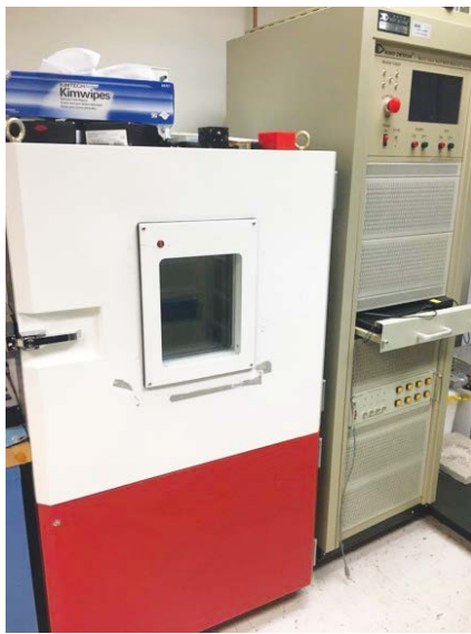
Figure 2. Guillotine test and highly accelerated life test (HALT) equipment used for MEMS shock testing.
