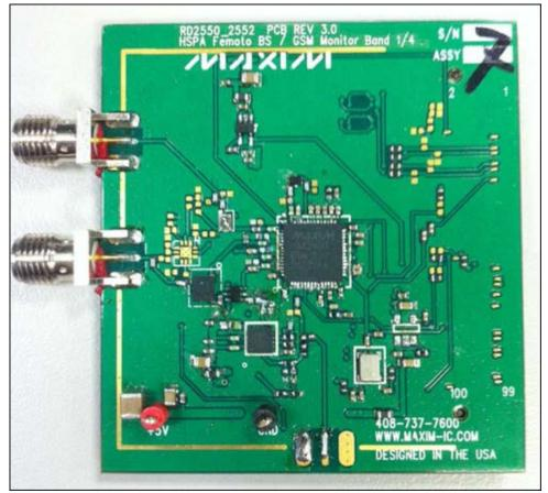
More detailed image (PDF, 1MB) Figure 3. Maxim femtocell base station reference design.
