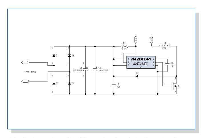
The 5W MR16 LED lamp circuit is shown using the MAX16820 LED driver. The LEDs shown are the LedEngin 5W WLEDs. (See page 10.)
