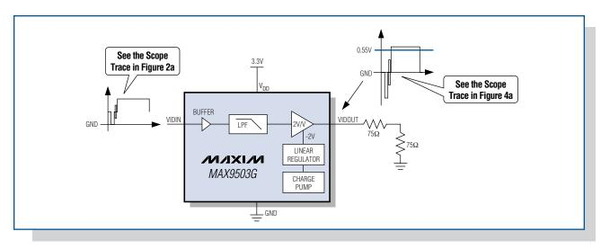
Figure 4. A 50% flat-field signal is processed through the MAX9503G application circuit.
