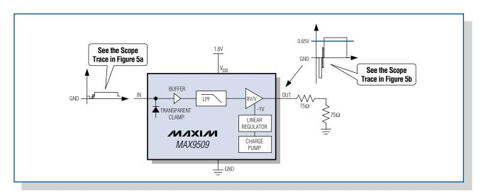
Figure 5. The MAX9509 1.8V application circuit processes a 50% flat-field signal, showing significantly reduced power consumption.
