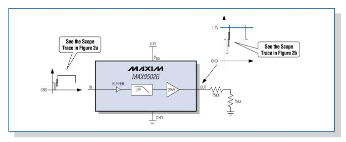
Figure 2. The MAX9502G application circuit shows the input and output of a 50% flat-field signal.
