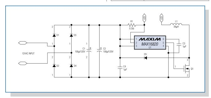
Figure 1. The 5W MR16 LED lamp circuit is shown using the MAX16820 LED driver. The LEDs shown are the LedEngin 5W WLEDs.
