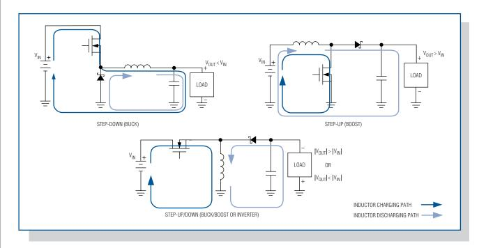
Figure 2. Buck, boost, and buck-boost compose the fundamental SMPS topologies.
