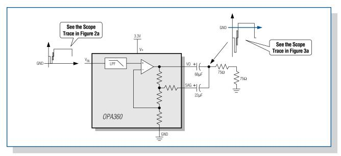
Figure 3. Given a 50% flat-field signal, the OPA360 application circuit minimizes power increase because the capacitors break the DC connection between the output and the load.
