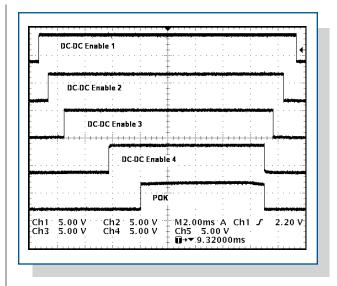
Figure 2. Beginning with DC-DC converter 1, the circuit of Figure 1 switches on three additional converters in sequence and generates a POK signal. Pulling the circuit's on/off input low removes the POK signal and switches off all four converters in reverse order.
