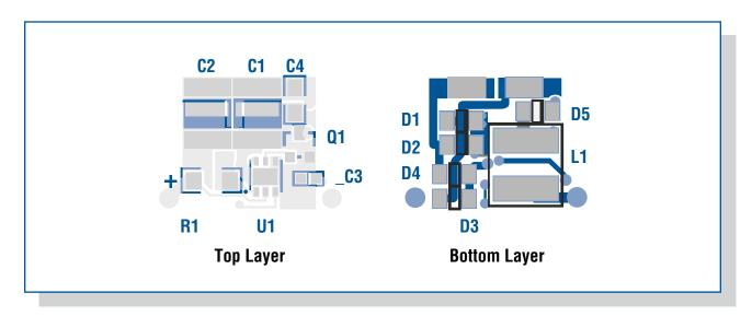
Figure 7. The LED+ and LED- DC-output connection pads can be seen on the 5W MR16 LED lamp driver PCB silk screen (top and bottom layers).
