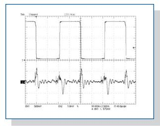
Figure 7. The MAX9509's output (bottom trace) is measured vs. time, taken with respect to a  $IV_{P-P}$  video signal. The spikes are  $1.4mV_{P-P}$ . The top trace is the voltage on the top plate of the charge pump's flying capacitor.
