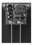
Figure 2. The LedEngin LED-based MR16 lamp has a very unique heatsink for dissipation of heat into the air. The MAX16820-based lamp driver board is placed just behind the heatsink.
