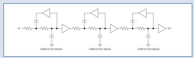
Figure 8. Previous generations of video filter amplifiers had 6-pole filters.
