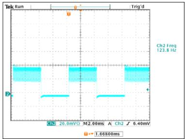
Figure 3b. LED current with an 85% eternal PWM duty cycle.
