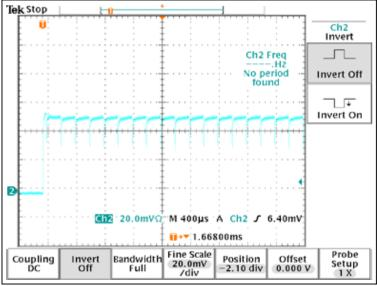
Figure 3c. Details of the external PWM effects.
