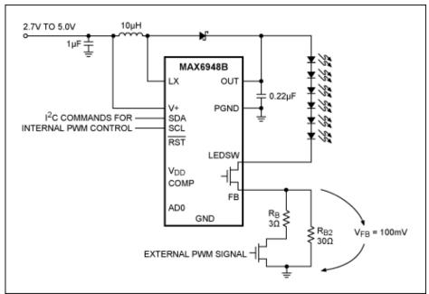
Figure 1. Circuit used to apply external PWM Control to the MAX6948B WLED driver. PWM from a microcontroller at 5kHz is applied with duty cycles from 0 to 100%.
