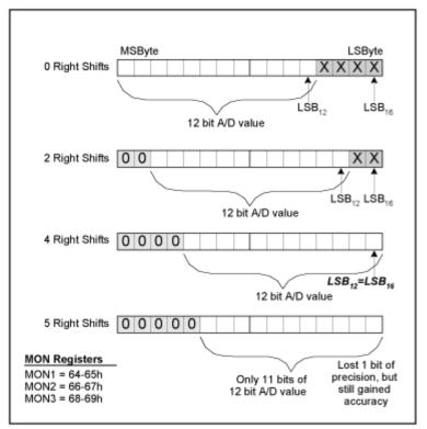
Figure 3. MON register right shifting examples.
