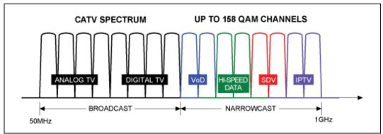
Figure 1. CATV spectrum includes broadcast and narrowcast services.
