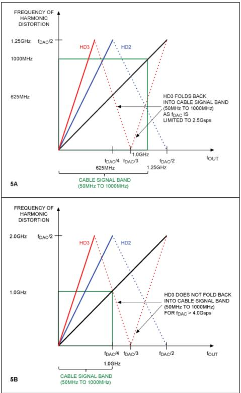
Figure 5. Synthesizing the cable band using a 2.5Gsps DAC (5A) and a 4Gsps DAC (5B).
