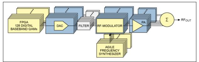
Figure 2. An older-generation analog upconverter combines multiple analog transmitters.
