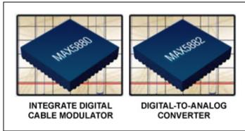
Figure 4. The MAX5880 is a 128-channel DUC and QAM modulator that drives the MAX5882 RF DAC.
