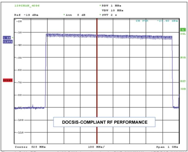
Figure 6. Cable RF spectrum of 128 QAM channels using the DUC (MAX5880) and RF DAC (MAX5882) chipset.
