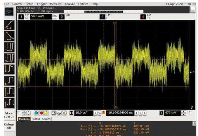
Figure 8. The output response of a -75 dBm pulse continuous wave input
