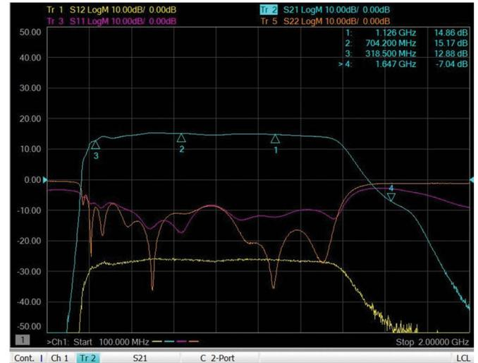
Figure 6. The S-parameter from the first stage to the final stage's ADL5513 input in a direct through path.
