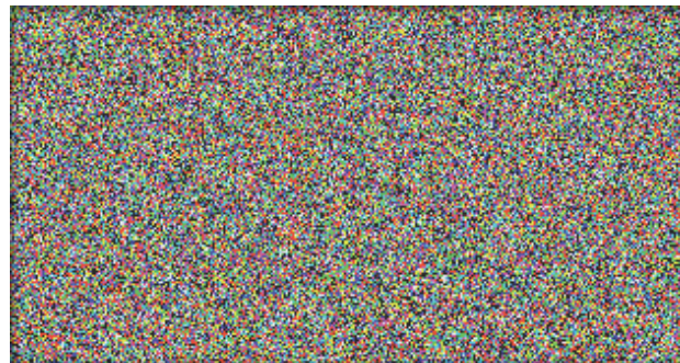
Figure 2. A sample of original content and HDCP snow noise caused by a HDCP failure.
