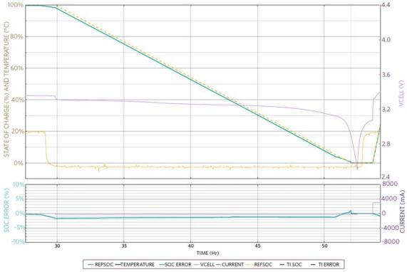
Figure 6. The SOC error remained under 2%, even at -5°C.
