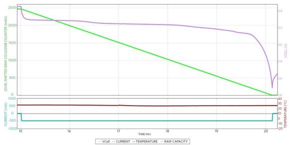
Figure 1. A typical discharge curve of an LFP battery.
