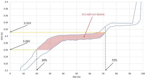
Figure 7. The OCV-SOC curve for an LFP cell with the OCV keep-out region. To prevent incorrect learning, this region is not used to calculate full capacity.
