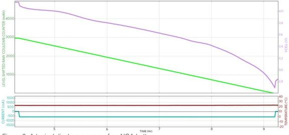
Figure 3. A typical discharge curve of an NCA battery.
