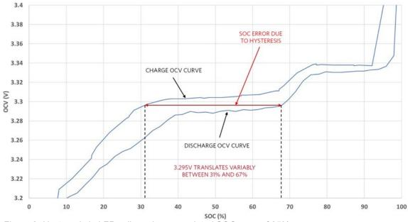
Figure 2. Hysteresis in LFP cells and an associated SOC error of 35%.
