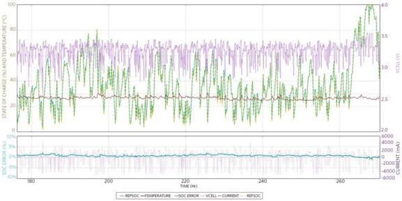
Figure 5. Accurate fuel gauging was achieved during the complex case of continuous use without reaching full or empty for more than a week. The error remained under 2%.
