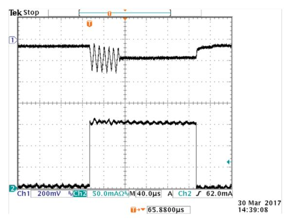
Figure 5. Noise during transition between modes.
