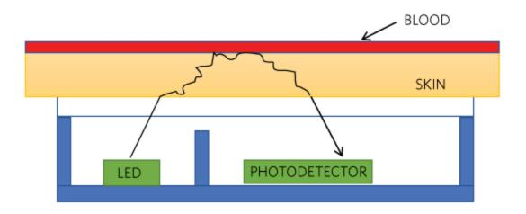
Figure 2. PPG signal using an LED and a photodiode.
