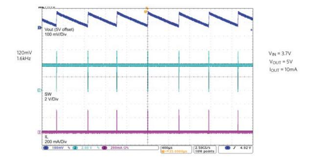
Figure 4. Burst mode voltage ripple of a boost converter with 10mA load current.
