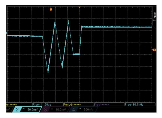
Figure 7. Slow response to load transients of a single-pulse duration.
