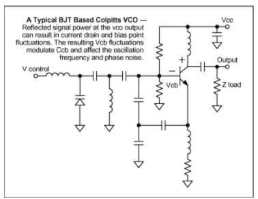
Figure 1. Signal power reflected at the output of this Colpitts VCO can produce fluctuations in the current drain and bias point. As a result, Vcb fluctuations in the transistor modulate Ccb, affecting the oscillator frequency and phase noise.
