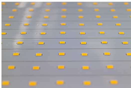
Figure 2. A detailed view of a full-array backlight LED panel.
