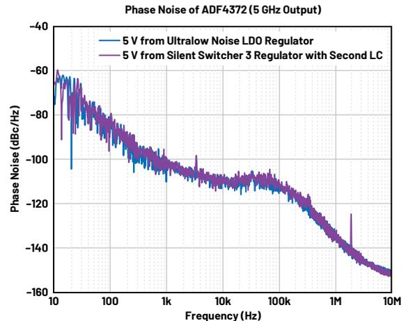
Figure 5. A comparison of the ADF4372 phase noise with 5 V from ultralow noise LDO regulator (LT3045) and the Silent Switcher 3 regulator (LT8625S) with a second LC filter.
