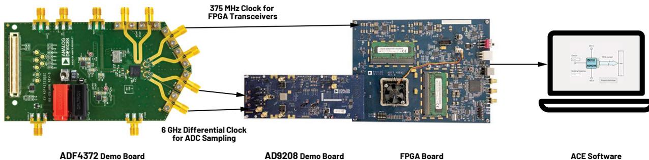
Figure 7. A detailed structure of the advanced ADC system under study.
