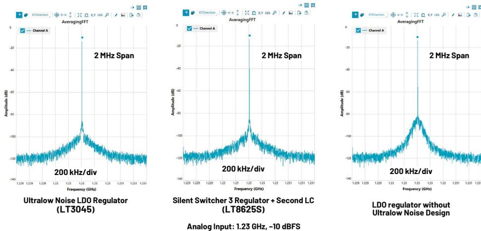
Figure 9. An average FFT result of ADC output signal under different power supplies for ADC sampling clock (Silent Switcher 3 regulator with second LC filter, LDO regulator without ultralow noise design).
