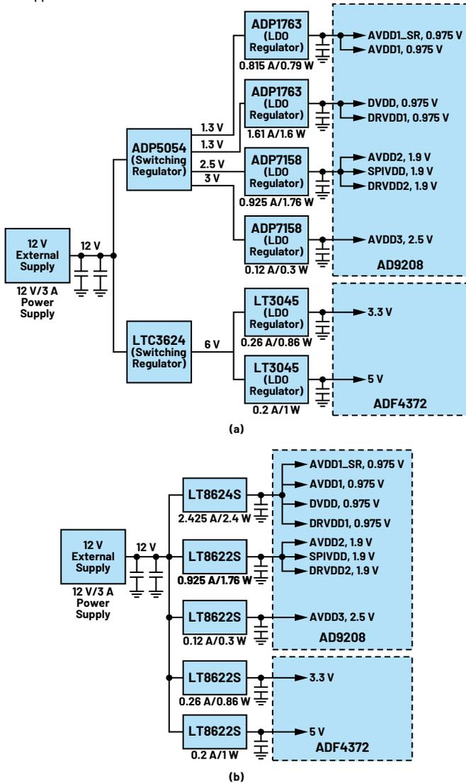
Figure 11. A comparison of the original and new power tree of ADC system (AD9208 + ADF4372): (a) original power tree (2-stage Buck + LDO regulator solution); (b) new power tree (single-stage solution based on Silent Switcher 3 technology).
