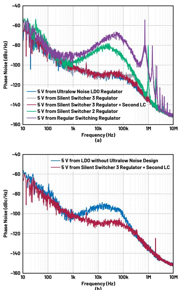
Figure 6. Phase noise of PLL clock (ADF4372) under different power supplies: (a) phase noise of ADF4372 (5 GHz Output); (b) phase noise of ADF4372 (5 GHz output).
