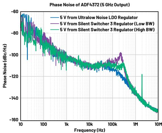
Figure 3. Impact of the Silent Switcher 3 regulator control bandwidth on phase noise of a high performance PLL.
