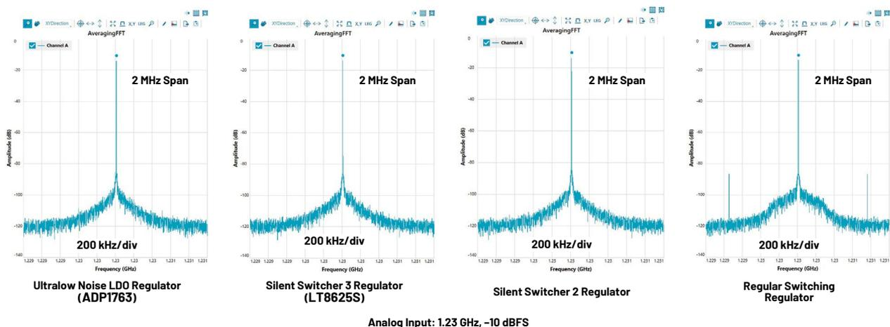
Figure 10. An average FFT result of ADC output signal under different power supplies providing AVDD1 (ultralow noise LDO regulator, Silent Switcher 3 regulator, Silent Switcher 2 regulator, and regular switching regulator).
