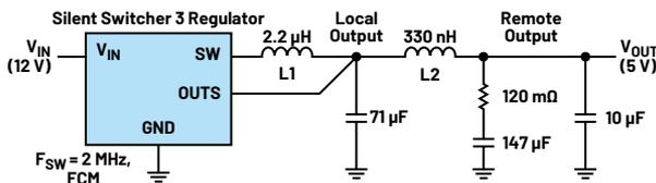
Figure 4. A circuit diagram of the Silent Switcher 3 regulator with a second LC filter to provide 5 V for the PLL.
