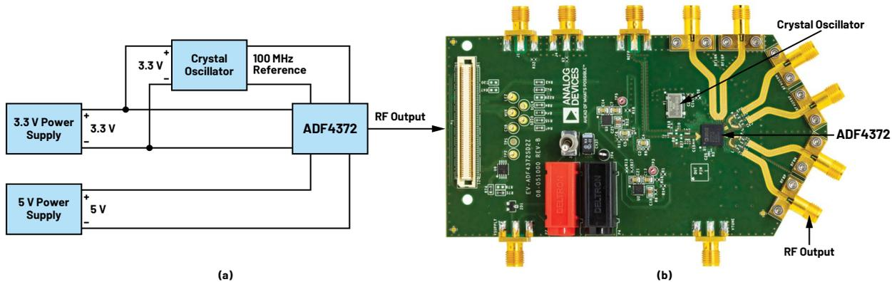
Figure 1. (a) A detailed power supply structure of ADF4372; (b) A demo board of the ADF4372.
