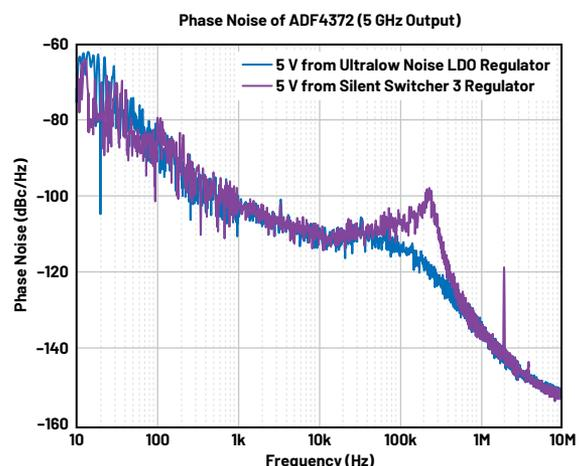
Figure 2. Baseline comparison of phase noise with 5 V from ultralow noise LDO regulator (LT3045) and Silent Switcher 3 regulator (LT8625S).
