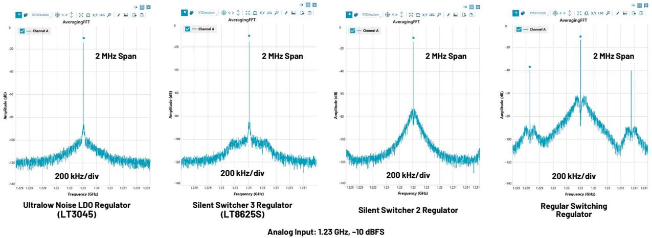
Figure 8. An average FFT result of ADC output signal under different power supplies for ADC sampling clock (ultralow noise LDO regulator, Silent Switcher 3 regulator, Silent Switcher 2 regulator, and regular switching regulator).
