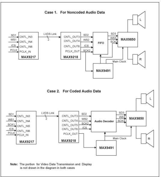
Figure 6. Implementation of audio replay in panel side.
