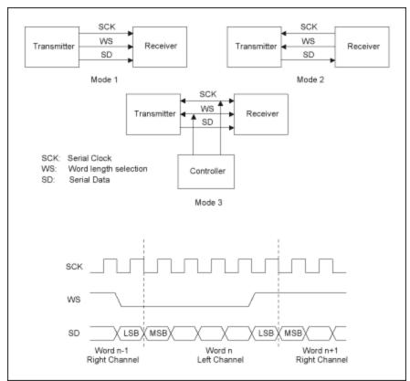
Figure 3. I<sup>2</sup>S interface configuration and timing.
