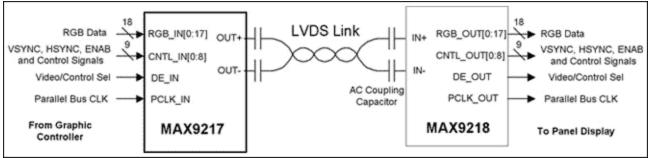
Figure 1. Video link setup with the MAX9217/MAX9218.
