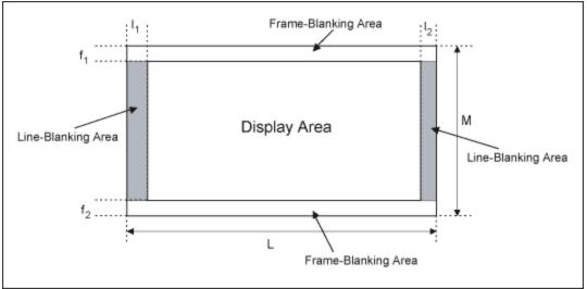
Figure 5. Line blanking and frame blanking.
