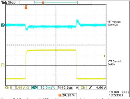
Figure 2. Waveforms of VTT and load current during a step load transient.
