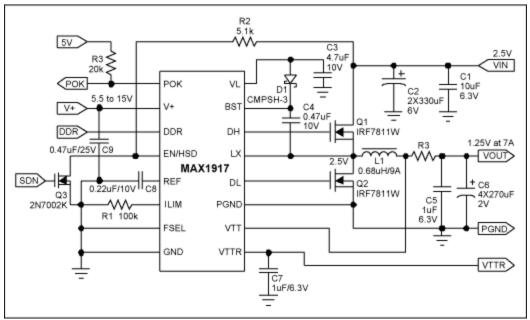
Figure 3. Schematics of VTT supply with output droop.
