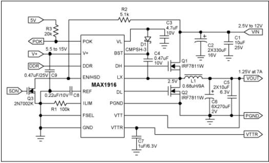
Figure 1. Schematic of 1.25V/7A VTT supply.
