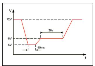
Figure 2. Typical vehicle cold crank voltage shape.
