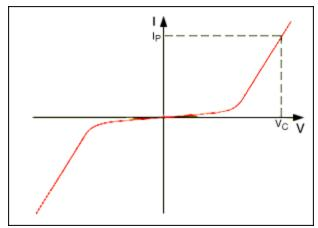
Figure 4. Typical varistor characteristic ( $V_C$  = clamping voltage @ peak pulse current,  $I_P$ ).
