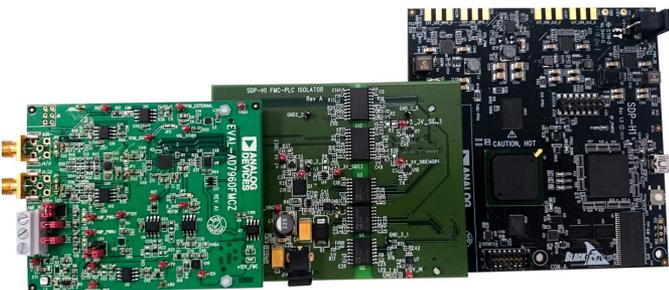
Figure 4. ADN4651 isolation circuit for AD7960 and SDP-H1.
