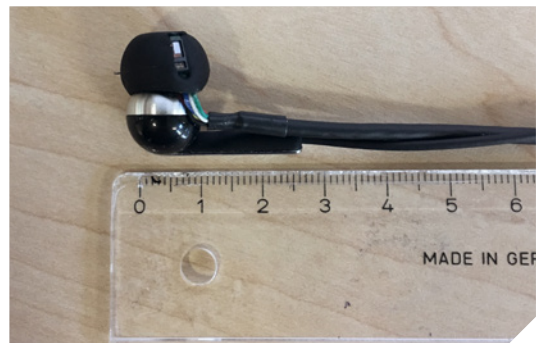
Figure 1. Test system with an integrated optical sensor and accelerometer with scale shown for comparison.
