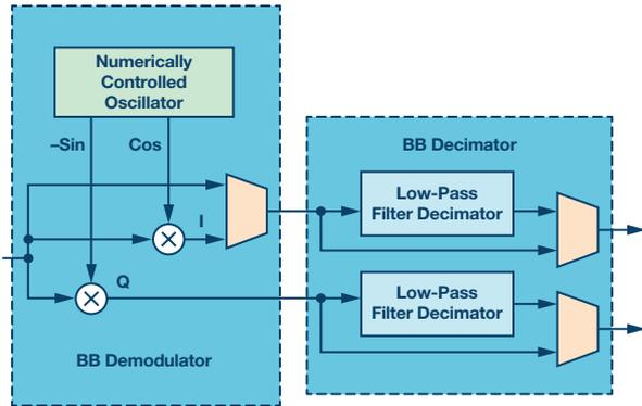
Figure 3. Digital demodulator block diagram.
