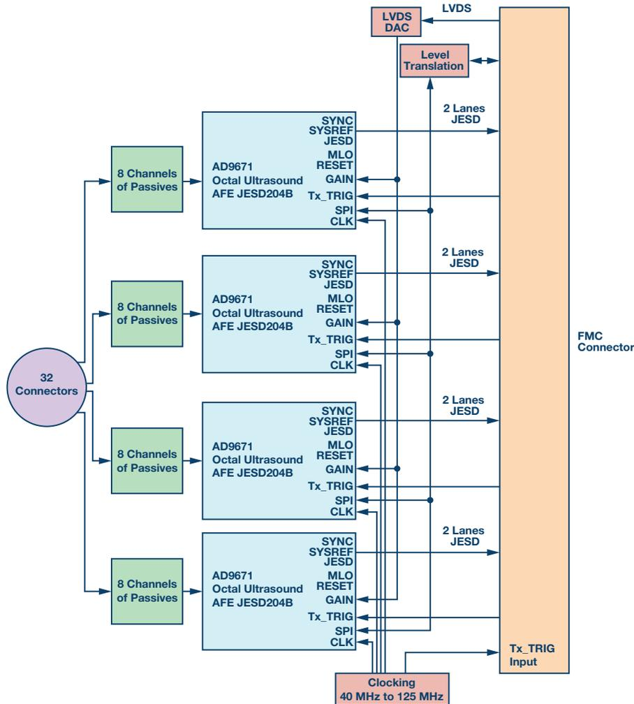
Figure 4. Top level schematic diagram of the receiving circuit.
