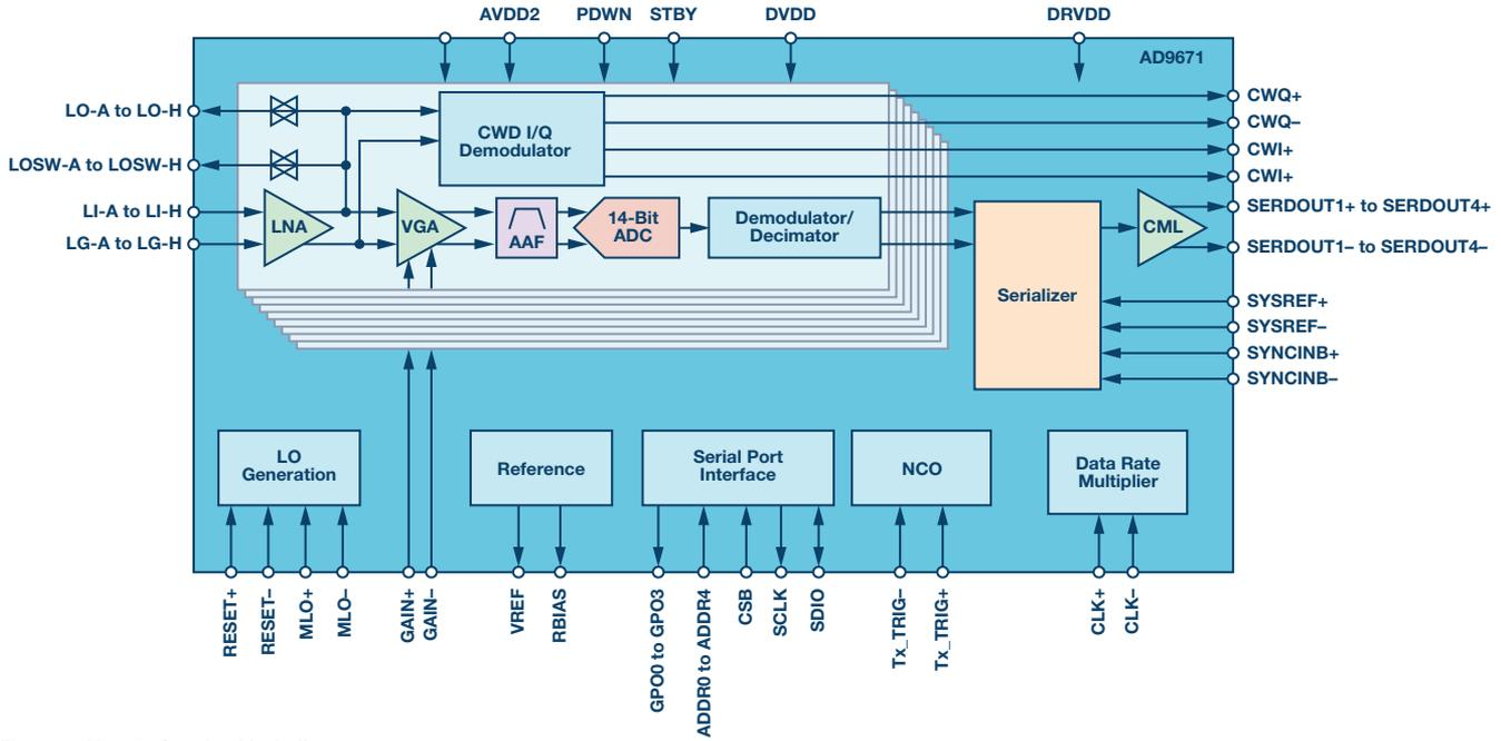
Figure 2. AD9671 function block diagram.
