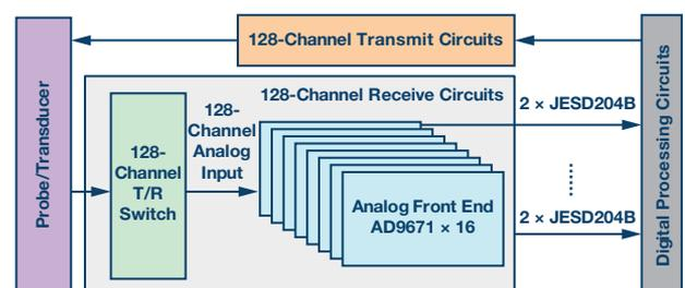
Figure 1. 128-channel ultrasound system block diagram.
