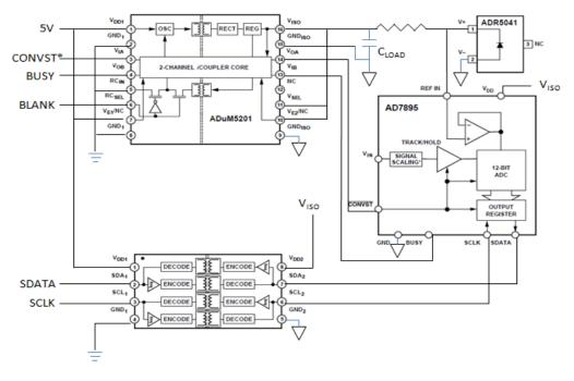
Figure 1. Isolated Low Noise ADC Circuit
