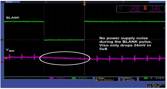
Figure 4. Full Operation with a 10 mA Load and 24 mV Supply Sag Due to the BLANK Pulse
