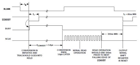
Figure 2. System Timing Diagram
