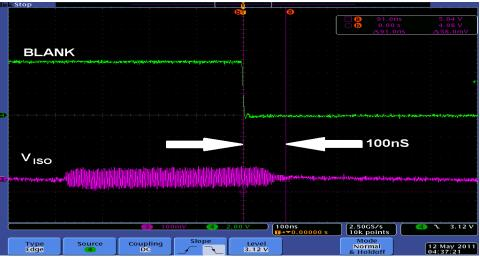
Figure 3. Delay from the BLANK Pulse to the End of the Power Supply Noise
