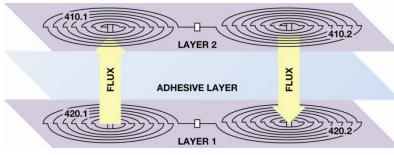
Figure 5. isoPower Transformer Configuration
