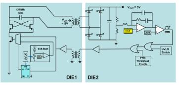
Figure 2. Schematic for Isolated Power Transfer Using Microtransformers
