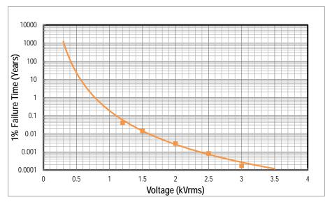
Figure 4. High Voltage Lifetime for isoPower Products
