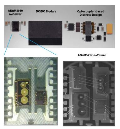
Figures 1. (a) Size Comparison of Various Isolated Power Implementations; (b) Inside Look of ADuM5010, a 150 mW Fully Integrated Dc-to-Dc Converter; (c) Inside Look of ADuM521x, a Dual Channel Isolated with Integrated Dc-to-Dc Converter
