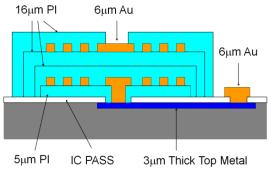
Figure 3. Cross Section of isoPower Transformers
