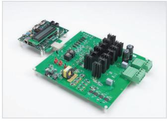
Figure 5. Analog Devices isolated inverter platform with fully featured IGBT gate drivers.
