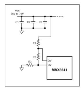
An alternate method used in the application circuits for setting the over-voltage and under-voltage trip points is demonstrated in **Figure 2**. Use  $36.5k\Omega$  for the bottom resistor (R3). R2 and R1 are calculated as follows:
