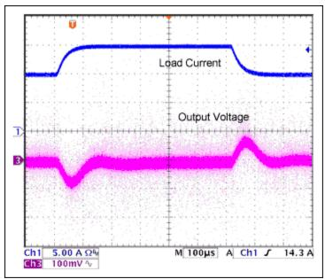
Figure 4. Output voltage deviation for step load increase and decrease. Load current slew rate is approximately  $0.1/\mu S$ .
