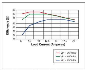
Figure 3. Converter efficiency vs load current.
