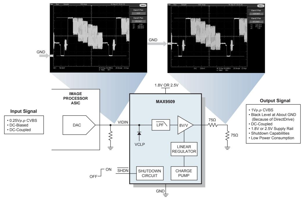
Note: Video DACs with a  $1V_{P-P}$  output signal can work in this configuration if the DAC's output terminating resistor is scaled down.
