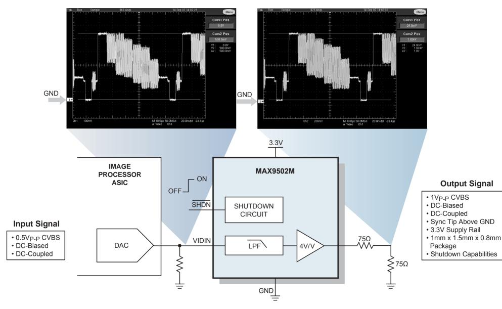
Note: This solution is not recommended if the design requires AC-coupling capacitors on the video output line; if this is the case, designers should seek a different solution.
