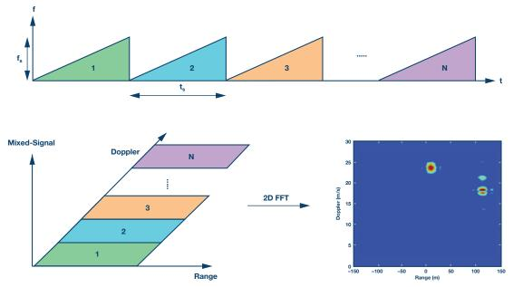
Figure 5. Range and doppler frequencies using 2D Fourier transform.
