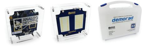
Figure 1. Demorad 24 GHz radar platform solution.
