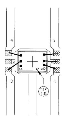
NOTE: MUST USE NON-CONDUCTIVE EPOXY
