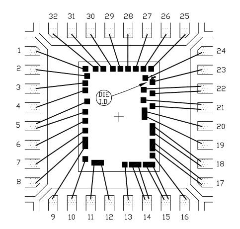
\*PINS5-12 HAVE SAME POTENTIAL (CONNECTED). \*PINS13-17 HAVE SAME POTENTIAL (CONNECTED). \*PINS18-22 HAVE SAME POTENTIAL (CONNECTED).
