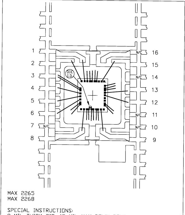
8 MIL THICK DIE, 15 MIL MAX DOWN BOND WIRES,
