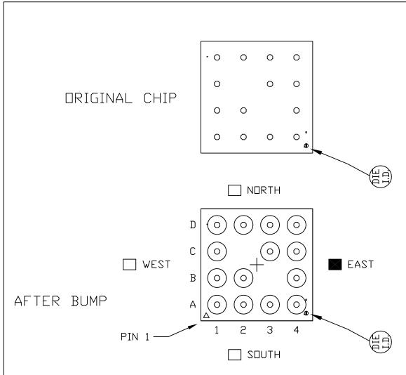
SELECT THE BOX INDICATING THE WAFER FLAT SIDE WITH RESPECT TO PIN 1.
