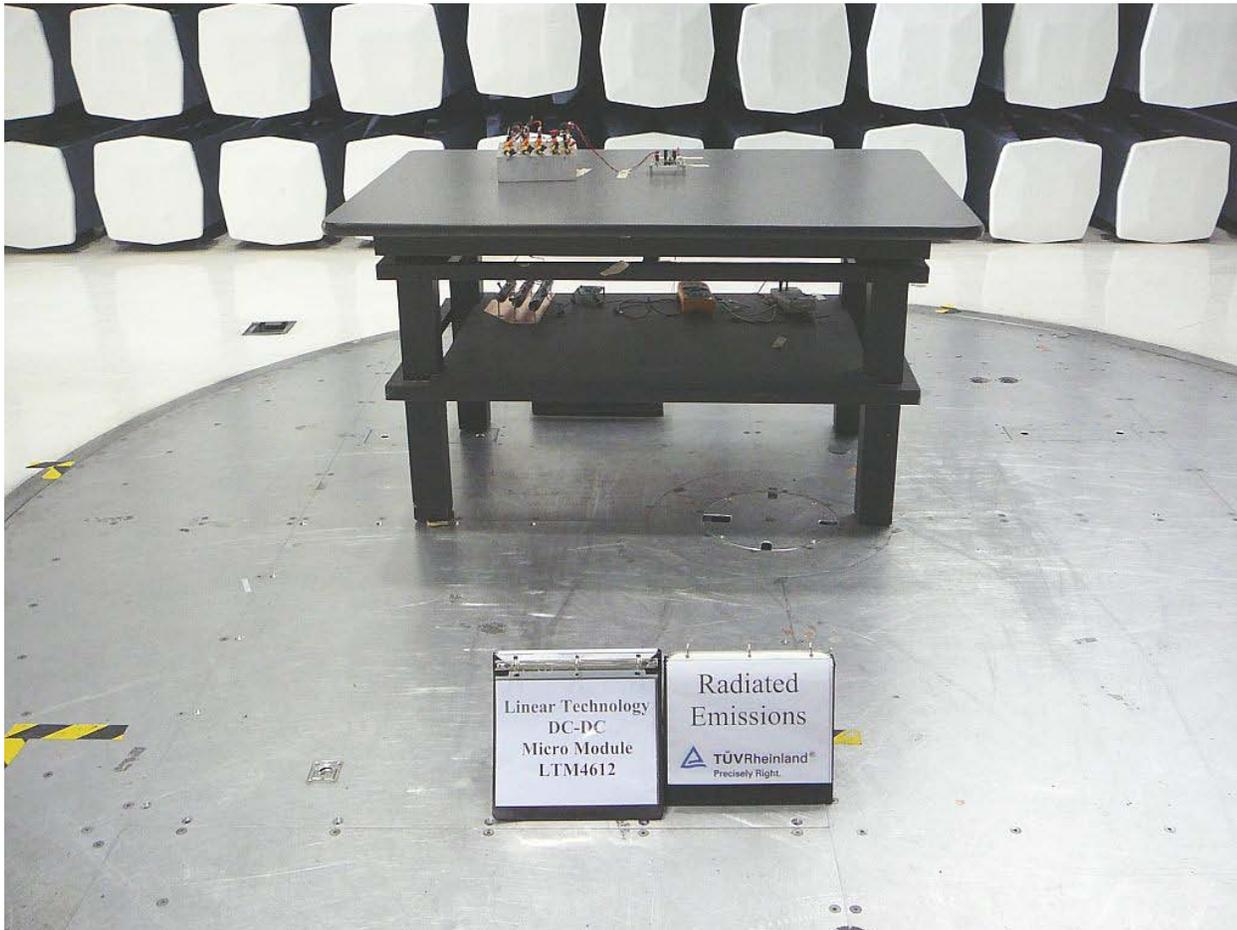
Figure 5 – Radiated Emissions 30 - 1000 MHz Test Setup – Load 2 – Front
