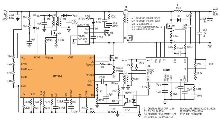
Figure 9. 150V-400V input, 12V/16.7A output isolated forward converter
