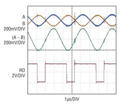
Figure 6. Duty cycle of competitor asymmetrical receiver with ±200mV 600kbps input signal
