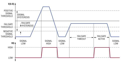
Figure 4. Failsafe window comparator operation
