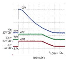
Figure 6. MIL-STD-1275D 100V/500ms surge test
