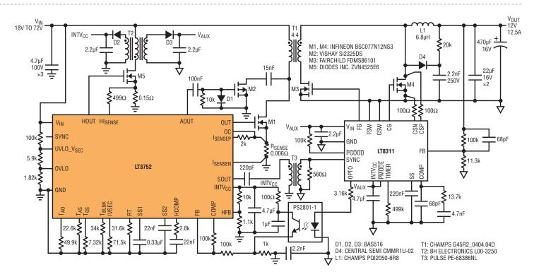
Figure 7. 18V–72V input, 12V at 12.5A output forward converter
