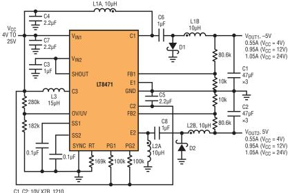
LT8471 500kHz ZETA AND 2L INVERTING CONVERTERS **GENERATES ±5V OUTPUTS WITH LOW OUTPUT RIPPLE**
