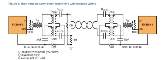
produce  $200\mu$ H. This has the additional benefit of forming virtual center-tap connections, which are useful for common-mode biasing and decoupling functions.
