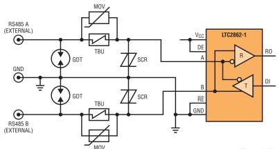
GDT: BOURNS 2031-42T-SM; 420V GAS DISCHARGE TUBE TBU: BOURNS TBU-CA085-300-WH; 850V TRANSIENT BLOCKING UNIT MOV: BOURNS MOV-7D391K; 390V 25J METAL OXIDE VARISTOR SCR: BOURNS TISP4P035L1NR-S; 35V BIDIRECTIONAL THYRISTOR Figure 9. Network for IEC Level 4 protection against surge, EFT and ESD plus ±360V overvoltage protection
