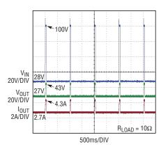
Figure 7. MIL-STD-1275D 100V/50ms surge repeated five times
