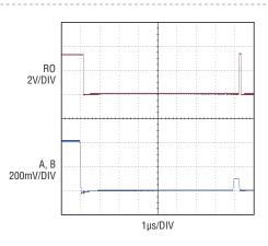
Figure 8. Competitor asymmetrical receiver responding to +100mV noise pulse on -200mV differential input
