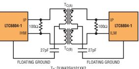
Figure 6. Daisy-chain isoSPI link for same-board interconnections
