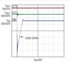
Figure 8. Positive input spike
