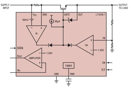
Figure 5. Simplified block diagram of the LT4356
