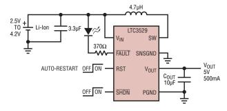
Figure 2. Li-Ion to 5V synchronous boost converter
