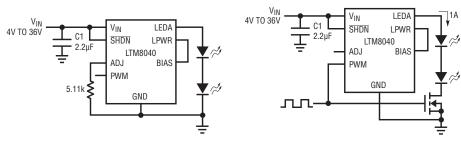
Figure 3. Control the LED current with a single resistor from ADJ to ground
