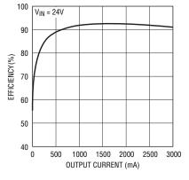
Figure 3. The LTM8025 boasts high efficiency.
