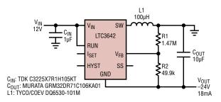
Figure 5. Generating a negative 24V output voltage from a positive 12V input voltage
