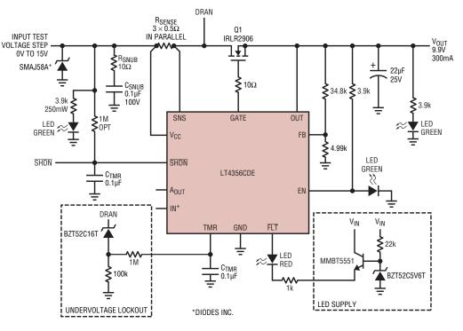
Figure 7. Schematic of a modified DC1018A evaluation board
