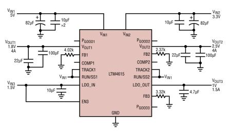
Figure 2. Very few components are required for a triple independent input (5V, 3.3V, 1.5V) to triple output (1.8V, 2.5V, 1V)  $\mu$ Module regulator design.
