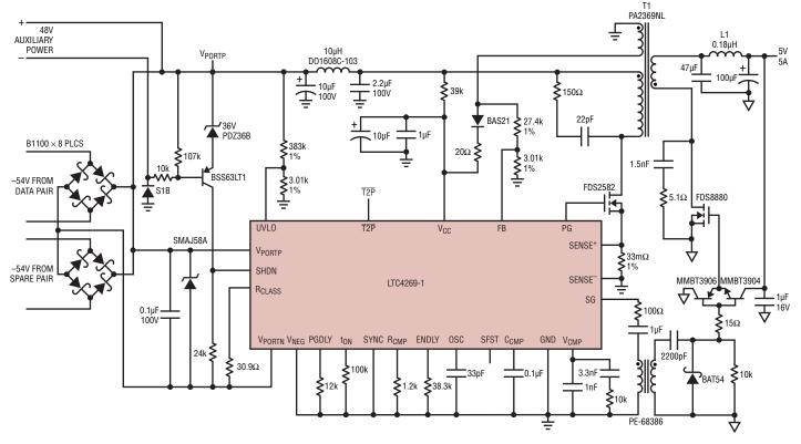
Figure 1. LTC4269-1-based synchronous flyback converter
