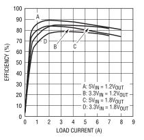
Figure 2. LTM4616 efficiency: dual output
