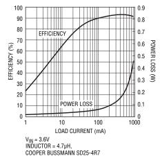
Figure 3. Efficiency for the circuit in Figure 2
