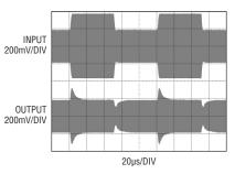
Figure 7. Measured analog control loop circuit response to 6dB step changes in input signal amplitude for  $C_F = 1000 pF$
