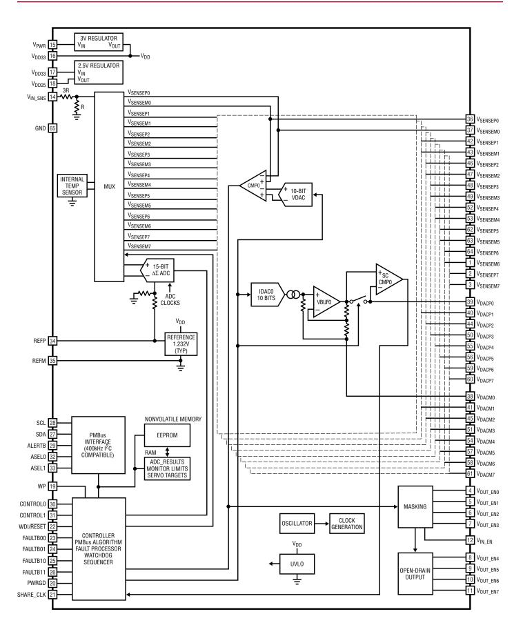
Figure 4. Block diagram of the LTC2978
