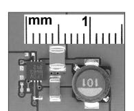
Figure 2. The solution size of LTC3642-3.3/5 in a 3mm × 3mm DFN package
