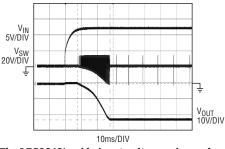
Figure 6. The LTC3642's wide input voltage swing makes it suitable for generating a negative output from positive input voltage.
