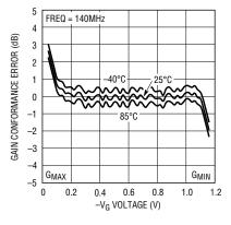
Figure 4. LTC6412 gain conformance error vs control voltage over temperature
