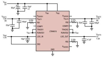
Figure 3. Single switching regulator input (5V) and single linear regulator input (1.5V) to triple output (1.8V, 2.5V, 1V)  $\mu$ Module regulator design
