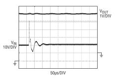
Figure 1. The LTC3642 continues to regulate the output despite a >45V spike on the input.
