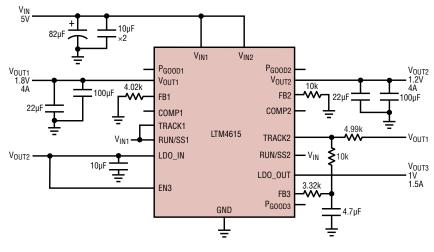
Figure 11. Output voltage tracking design example
