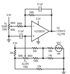
Figure 12. Thermistor-based application circuit for static gain adjust and temperature gain slope compensation. Adjust R1 and R2 as needed and route output to  $-V_G$  control terminal of the LTC6412.
