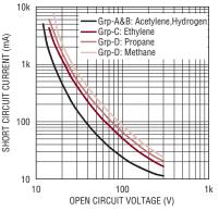
Figure 4. Resistive circuit spark ignition curves
