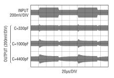
Figure 8. Measured analog control loop response to 6dB step changes in input signal amplitude over a range of  $C_F$  values
