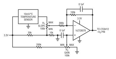
Figure 10. Application circuit for static gain adjust and temperature gain slope compensation using a PTAT temperature sensing IC. Adjust R1 and R2 as needed and route output to  $-V_G$  control terminal of the LTC6412.
