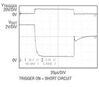
Figure 9. Overcurrent fault operation
