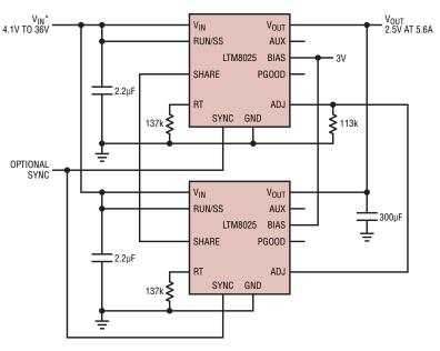
\*RUNNING VOLTAGE RANGE. PLEASE REFER TO APPLICATIONS INFORMATION SECTION FOR START-UP DETAILS NOTE: SYNCHRONIZE THE TWO MODULES TO AVOID BEAT FREQUENCIES, IF NECESSARY. OTHERWISE, TIE EACH SYNC TO GND
