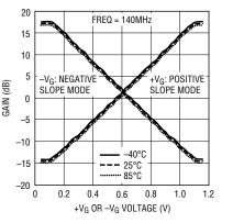
Figure 3. Differential gain vs control voltage over temperature for the LTC6412
