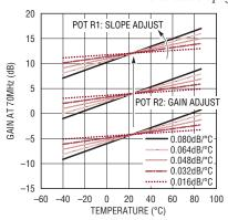
Figure 11. Gain vs temperature performance characteristics of the PTAT sensor based circuit shown in Figure 10
