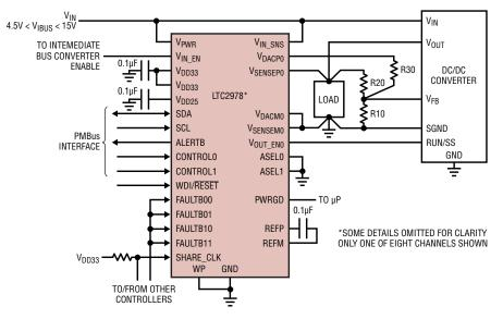
Figure 1. Octal power supply controller with PMBus communication. One channel is shown.
