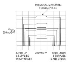
Figure 2. The LTC2978 offers flexible sequencing and precision margining.
