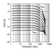
Figure 2. LTC6412 gain vs frequency over gain control range
