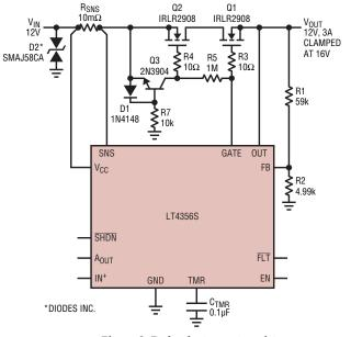
Figure 6. Redundant pass transistors
