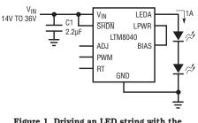
Figure 1. Driving an LED string with the LTM8040 is simple—just add the input capacitor and connect the LED string
