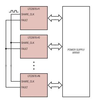
Figure 3. Multiple LTC2978s can be cascaded using only two connections.
