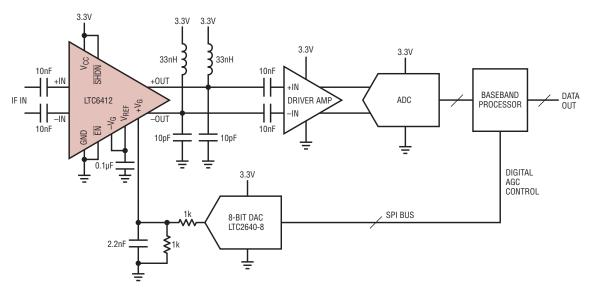
Figure 9. Digital control loop application circuit at IF = 240MHz. LTC6412 bypass capacitors to ground omitted for clarity.
