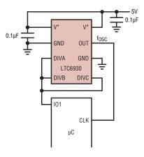
Figure 1. The LTC6930 clock configured as a 2speed clock, slow and fast clock speeds are set via one I/O pin on a microprocessor
