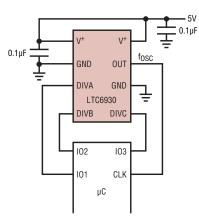
Figure 2. Fine control of the the LTC6930's frequency via three microprocessor I/O pins
