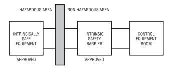
Figure 2. Isolation/protective barrier location
