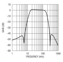
Figure 1. Filter response for a 15kHz-150kHz passband
