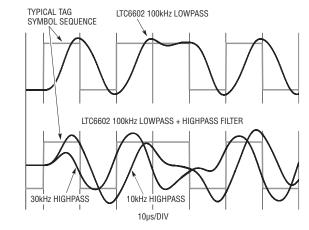
Figure 3. Filter transient response to a tag symbol sequence
