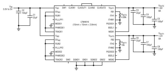
Figure 1. Dual output LTM4616 for a single 3.3V to 5V input, independent 1.8V and 1.2V outputs at 8A each
