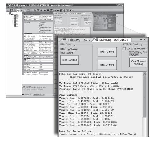
Figure 5. The LTC2978 comes with free software that allows easy data monitoring and cofiguration. The data log shows monitor readings just before a failure for debugging analysis.
